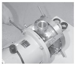
Figure 22 - Remove body nuts (4)
