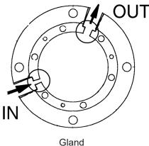
**NOTE:** These are 1/4-inch pipe nipples, but the IN hole is smaller than the OUT hole to prevent over-pressurizing (Figure 4).
